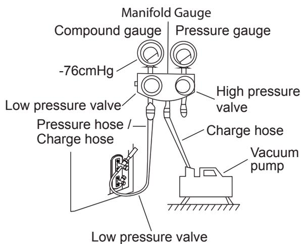
1. Connect the charge hose of the manifold gauge to service port on the outdoor unit's low pressure valve.
